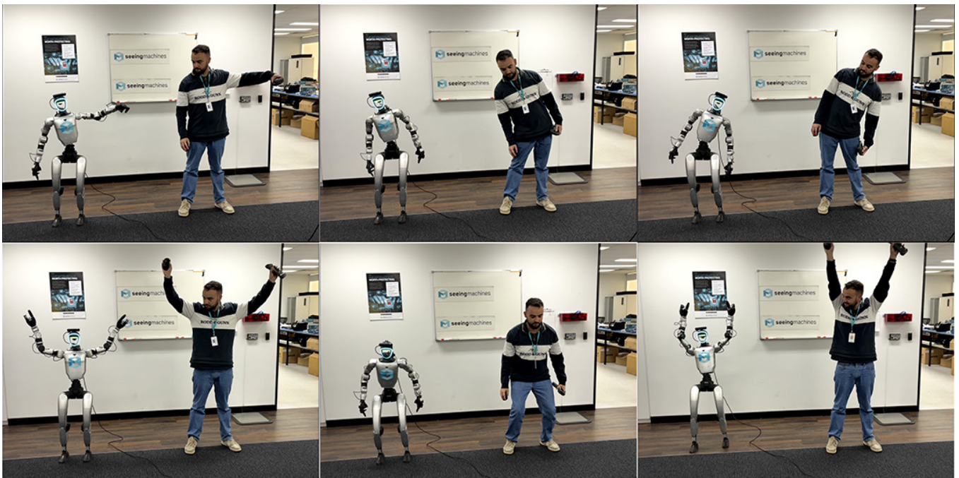
Figure 5. Real-time Teleoperation of Unitree G1 using Seeing Machines' HMR on NVIDIA Jetson Thor.
