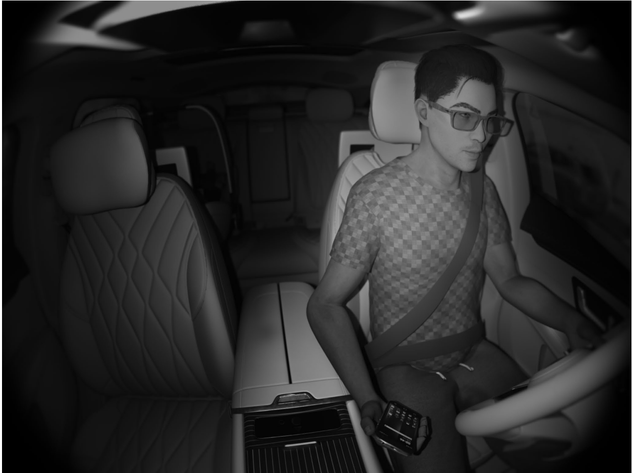
Above: Lens model applied. Here a fisheye lens with finite aperture is used. The image now has accurate distortion, depth-of-field blurring and attenuation effects.
