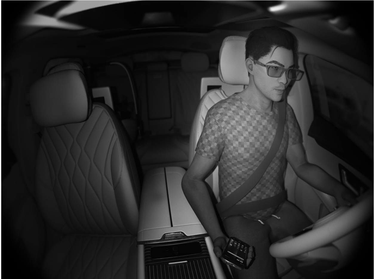
Above: Sensor model applied. In this final stage of the camera simulation, the image is sampled at the resolution and bit-depth of the image sensor, with sensor-specific and temperature dependent noise properties.
